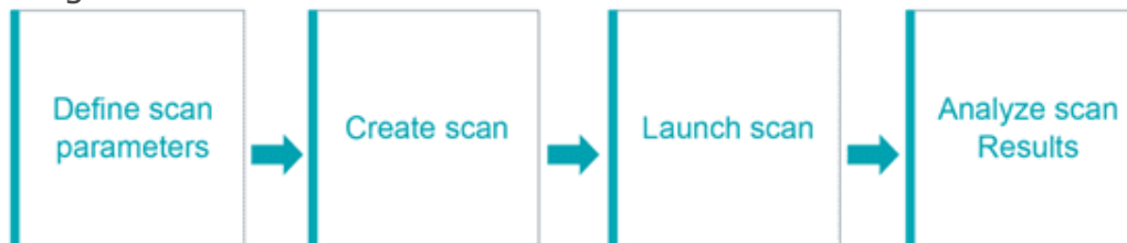
Figure 3.10: Nessus Scanning Process
