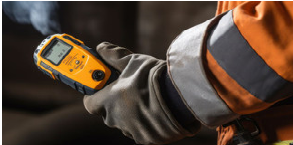
Figure 3 Manual gas level monitoring using handheld device in Hazardous Environment (William Kimmell, 2023)
