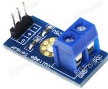
Figure 12 DC voltage level sensor (Datasheet. 2022).
